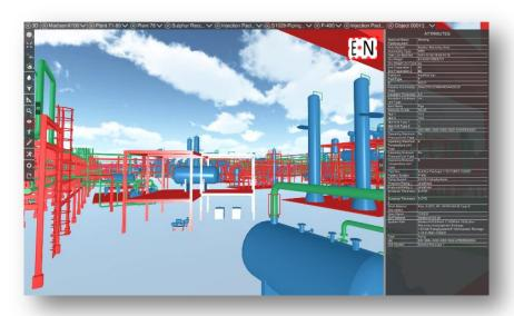
Universal Plant Viewer is capable of viewing an entire plant such as a complete oil refinery (or even larger) via the internet. Data, drawings and documentation are packaged together using Universal Plant Viewer into either a web based format or a PDF document for use with Adobe Acrobat Reader. This removes the need to buy or install specialist software — most PCs already have a suitable web browser or Acrobat Reader already installed.
